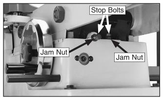
Figure 48. Infeed table positive stop bolts.
